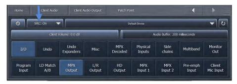
◆ The client software recognizes any audio output devices (speakers, headphones, sound cards) installed on the remote control PC, and makes them available in the Output Device drop-down menu
