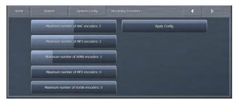
♦ Selecting the Apply Config button will places any changes you have made into effect. This will take your station off the air and disconnect all streams for a few seconds.
