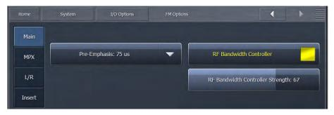
◆ Enabling the RF Bandwidth Control can tightly control the RF bandwidth to reduce multipath problems. The Strength slider determines the amount of control applied.
