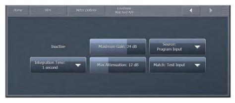
♦ Source audio and Match audio can both come from either the Program Input to the HD core or from the Test Input as selected in the Test Input Menu.
