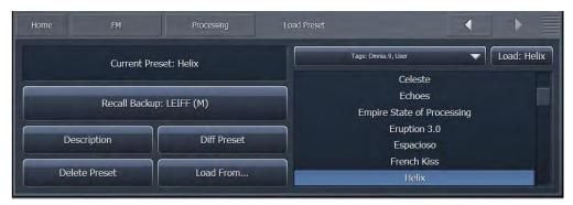
Highlighting a preset from the list places it in the Load button. Selecting the Load button puts that preset on the air and moves it up to the Current Preset position. The preset that was previously on the air will become the Backup Preset. You may also place a preset on the air from the list directly by double tapping it.
