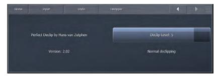
A setting of Level 5 the "normal" setting and recommended for most modern material which have been mastered with high levels of compression and clipping. If your station primarily plays source material that has been cleanly mastered, you may find lower settings are sufficient.
