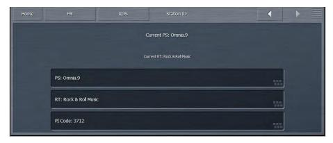
Typically, the PS field – an 8-character static display – contains the call letters of the station – for example. WOMN-FM. However, it is possible to program the PS field in such a way that it can provide a bit more information. Here are some ways to creatively use the PS field:
