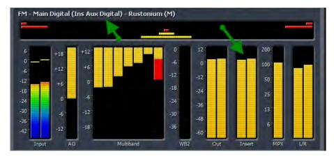
Whenever the Insert Mode is active, you will see an additional label at the top of the Processing Meters display indicating so. An additional set of Insert meters (which should be in perfect sync with the Out meters when the null is properly set) provides additional visual verification that the Insert Mode is active.
