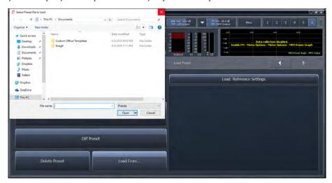
When using the Load Preset function, be aware that the preset will be loaded to the Current Preset position and will therefore immediately go on the air. Additionally, in order for the preset to appear in the list, you must save it using the Save Preset function.
