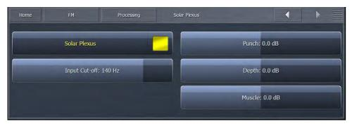
♦ When activated there are 3 adjustments to control the effect that can be set to reduce as well as boost the Punch, Depth and Muscle features of the effect as desired. When adjusting Solar Plexus, be sure to use speakers or headphones with good low bass response to avoid "overdoing it" with too much energy in the lowest octaves.
