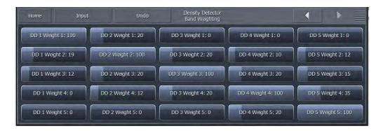
To put this concept into traditional processing terms, it is similar to "band coupling" in a multiband compressor, where all bands may operate completely independently of one another or may influence one another by way of coupling to varying degrees.
