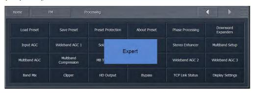
There are obviously additional buttons under "Processing", all of which are explained shortly. The "About Preset" button also has a simpler function of recording the originator of a processing preset, and providing a textual description and name of a preset. By default, each preset loads in the Basic mode
