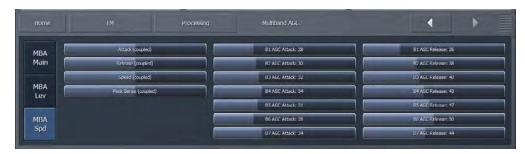
The Multiband Attack/Release section lets you control the Attack Speed and Release Speed of each band in the multiband AGC section.
