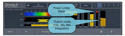
Controls for adjusting the Power Limiter are found in the FM> Processing> Power Limit menu.
