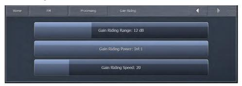
◆ The setting of the Gain Riding Range control affects the Input AGC only and determines the amount of available gain. Setting this control too high may provide too much room for low level audio to be raised up while not providing enough room to adequately attenuate higher input levels. Conversely, setting it too low may not provide enough gain to increase low incoming levels.
