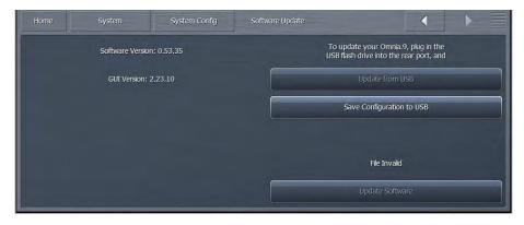
The update .pak file downloaded from the Omnia website must be used as-is and can be copied to the root of an external USB drive to update the unit locally or can be used by the NfRemote software to update the unit remotely.
