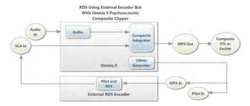
Be sure to enable the proper MPX input for RDS use (Input 1 or Input 2) in the RDS Mode menu, and set the MPX 2 Output control to the 19kHz Generator mode. The MPX 2 Output control can be found in the RDS Menu, the FM Processing Output menu, and in the main I/O menu.
