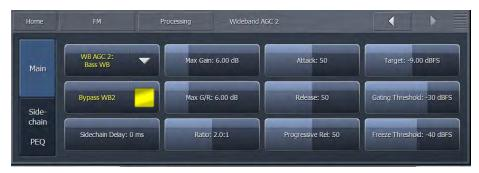
The Wideband AGC2 Main menu provides access to the Sidechain Delay, Maximum Gain, Maximum Gain Reduction, Ratio, Attack, Release, Progressive Release, Target, Gate Threshold and Freeze Threshold.
