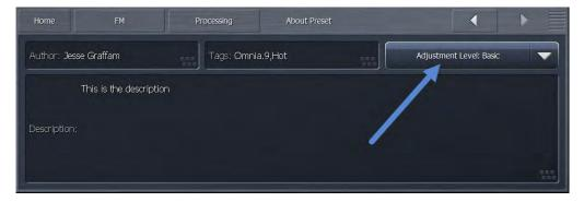
The choice of the "Adjustment Level" will determine how much finesse is made available to the operator, with "Basic" providing access to five controls to affect the main FM signal,
