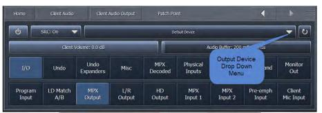
♦ The Client Volume slider controls the volume of the selected output devices on the remote PC. This control is duplicated on the top menu of the client software where it is available at all times.
