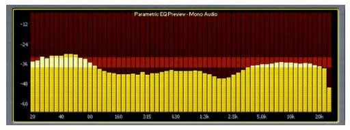
You will now be able to see the curve of the PEQ in the RTA display window. You can also view the curves of each band of the multiband compressor by selecting one of the Solo band buttons. Since the Solo bands relate to a dynamic section of the processing core, lowering the Averages slider will yield more of a "real time" view.
