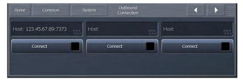
One example of how this can be used is for technical support. By creating an outbound connection, you are connecting to the support engineer's NfRemote computer which in turn allows them to control your Omnia.9.
