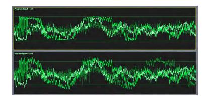
The second stage of Undo is a multi-band expander that is designed to restore dynamic range to audio that has been excessively compressed. Each of the five bands of the expander has a corresponding psychoacoustic dynamics detector and a peak detector that examine the peak levels of the incoming audio, and based upon that information plus the settings of the various controls, tells the expander how much dynamic range to restore to the audio.
