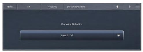
Dry voice is one of the most difficult waveforms to process cleanly, as the human voice is complex in nature and is typically asymmetrical in form. Stations that choose to process aggressively in an effort to maximize loudness may find that bare vocals come through with unacceptably high levels of audible distortion.
