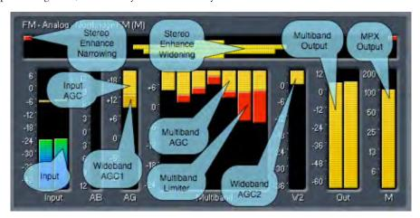
In the FM processing core, meters are provided for monitoring input levels, Input AGC, Wideband AGC1, Multiband AGC and Limiters, Multiband Noise Reduction, Multiband Stereo Enhancement, Wideband AGC2 and AGC3 sections, post-multiband output, MPX output, and individual left and right outputs. In the HD and Streaming cores, meters for the final look-ahead peak limiters and the final output of the processing core are added, while the MPX output and left and AGC output meters are eliminated.
