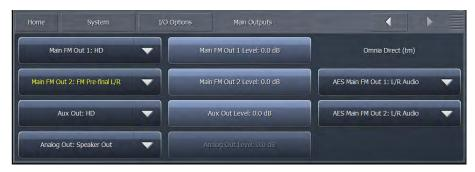
♦ The Main FM Out 1, Main FM Out 2, Aux Out, and Analog Out drop-down controls offer a choice of FM pre-emphasized or FM de-emphasized audio, audio from the HD-1, HD-2, and HD-3 processing cores (depending upon configuration) and audio from the Headphone, Speaker, and Aux monitor outputs.
