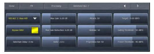
The Wideband AGC2 menu provides access to the Sidechain Delay, Maximum Gain, Maximum Gain Reduction, Ratio, Attack, Release, Progressive Release, Target, Gate Threshold, and Freeze Threshold.
