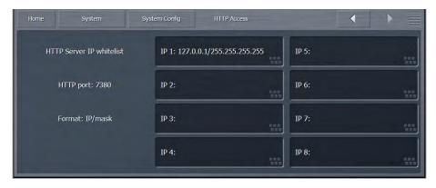
◆ Enter the IP address and subnet mask information using the following example as a guide: 192.168.1.0/255.255.255.0 (The beginning of the IP range followed by the subnet mask, separated by a forward slash).
