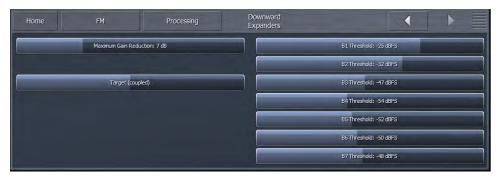
The Downward Expanders operate in a manner similar to a traditional "noise gate," and are useful for reducing unwanted background noise from less-than-perfect program material or from a noisy studio environment. The ratio of these expanders is 2:1.
