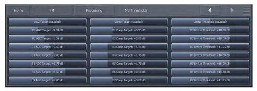
The AGC Target controls set the target output level of each band of the Multiband AGC. A lower setting provides a lower output level, while a higher setting provides a higher output level. These controls have a range between +12 and -12dB in one-tenth dB increments.
