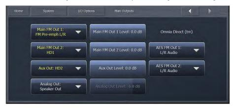
For example, the Main FM Out 1 might be set to "FM Pre-emph L/R" in order to output pre-emphasized audio for the main FM channel which will be de-emphasized later in the chain. Main FM Out 2 might be set to "HD-1" to route audio destined for the HD-1 path. Aux Out may be set to "HD-2" for audio being sent to the HD-2 path.
