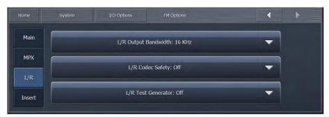
♦ The L/R Output Bandwidth slider performs the same function for the Left/Right outputs but with a choice of 15, 15.5, 16, or 16.5kHz.
