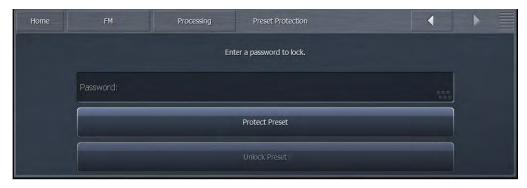
To password protect a preset, enter a password, click on "OK," and then on "Protect Preset." A warning dialogue box will appear. If your intention really is to protect the preset, select "Yes." The final step is saving the new, protected preset with a unique name in the Save Preset menu. Protected presets appear in green in the Load Preset menu. Remember not to accidentally leave an unencrypted version your preset in the Backup Preset slot!
