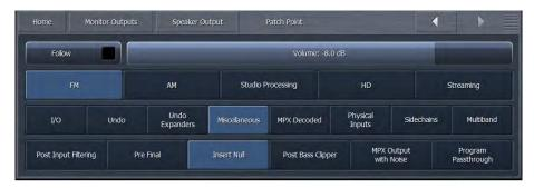
This patch point takes the audio routed through the "Pre-final L/R" output, adds the amount of compensation delay as set by the Insert Delay control, subtracts it from whatever is routed through the currently selected Input Source, and outputs the (hopefully!) nulled result.
