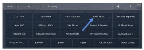
All of the processing controls and settings found in other processing cores (FM, HD, Studio, Streaming) are present here and function in exactly the same way, including the need to set the Adjustment Level under the About Preset tab.
