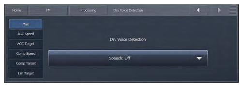
Dry voice is one of the most difficult waveforms to process cleanly, as the human voice is complex in nature and is typically asymmetrical in form. Stations that choose to process aggressively in an effort to maximize loudness may find that bare vocals come through with unacceptably high levels of audible distortion.
