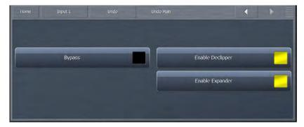
When selected, the **Bypass** control turns off both the de-clipper and the expander portions of Undo.
