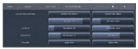
◆ Selecting the Update Time or Update Date sliders will refresh the time displayed on the sliders. Use the Set Hour, Set Minute, Set Second, Set Year, Set Month, and Set Day sliders to reflect the current time and date, then select Apply Time or Apply Date to put the new values you have set into effect.
