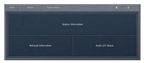
The **System Information** portion shows information about Omnia.9's operation, including CPU load, available RAM, power supply health, up time, and various software, firmware, and hardware versions.
