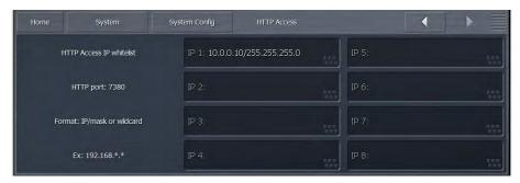
Using a web browser of your choice (and the actual IP address of your Omnia.9 to replace the sample address here), enter "http://192.168.1.1:7380". This will bring up the HTTP server home page which contains a link to the NfRemote software. Download, locate and install the software. Once installed, assign
