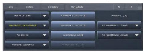
If you are using the composite outputs, levels are set in the System > I/O Options > FM Options menu.
